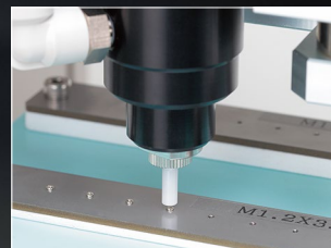
Tightens screws as small as M1.0.
