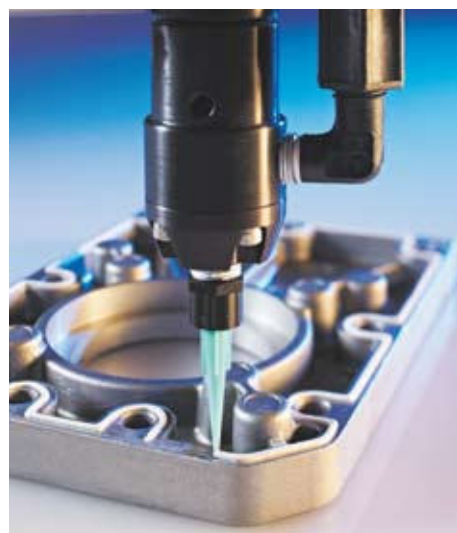
• Sigillatura TS5322, TS500R , serbatoio
